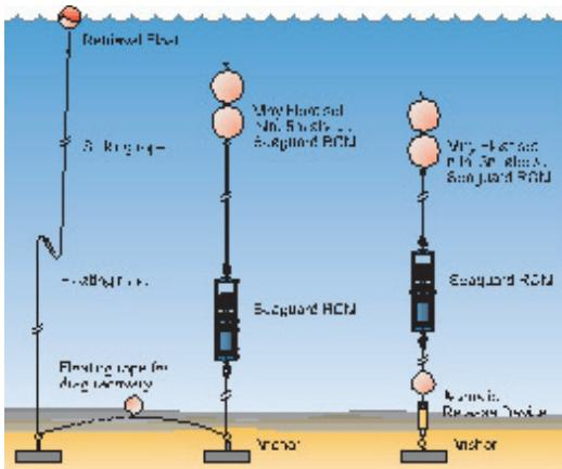
The most common way to use the SEAGUARD® RCM is in an in-line mooring configuration. As it operates under a tilt up to 35° from vertical, it has a variety of in-line mooring applications by use of surface buoy or sub surface buoy. The instrument is installed in a mooring frame that allows easy installation and removal of the instrument without disassembly of the mooring line.
