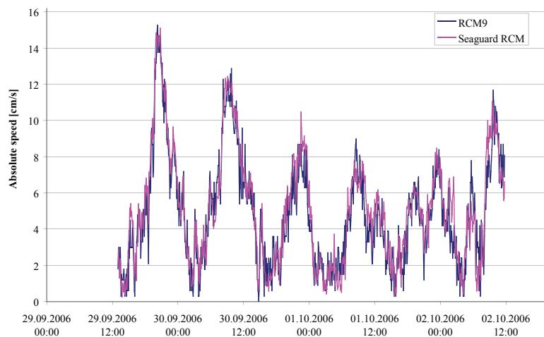
Comparision between data measured by a SEAGUARD® RCM (pink) and a RCM 9 (blue). The graph is showing absolute speed measured in a fjord outside Bergen, Norway.
